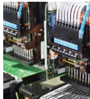
Dual mounthead carrier system.
