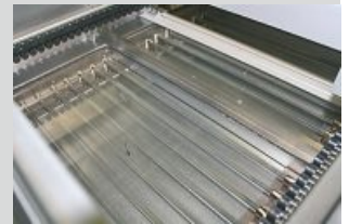
infrared preheat zone
